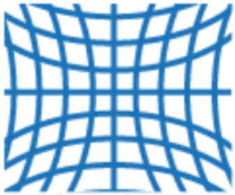
Pincushion distortion Positive radial displacement
