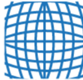
Barrel distortion Negative radial displacement
